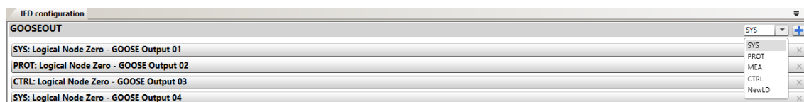
Figure 15. Configuration of GCBs in Different LDs.
