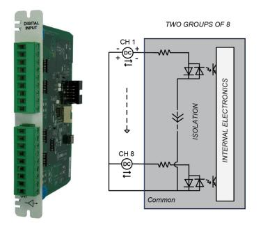
The MDI digital input module has 16 digital input channels organized as two groups of 8 with respective commons. It accepts bidirectional Voltage-Driven inputs and provides optically isolated input channels with field voltage ranges from 18 to 72V DC and 36 to 150V DC. Connections are via a pair of 9-way removable plugs to fixed card side sockets. This greatly simplifies panel build and allows for easy connection/disconnection of plant wiring.
