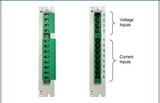
The MAC-020 is a high accuracy input module for AC metrics. It supports 3 AC voltage inputs and 4 AC current inputs.
