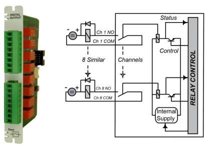
The MDO is an 8 channel digital output module with a single normally open contact per channel. Suitable for 125VDC operation
