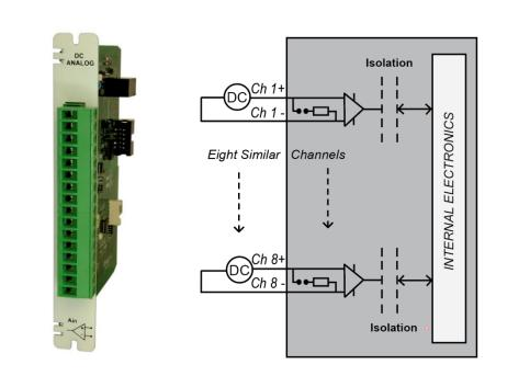
The MAI is an 8 channel DC analogue input module which provides the measurement options for 0-1V, 0-10V,  $\pm$  1V,  $\pm$  5V,  $\pm$  10V,  $\pm$ 20mA and 4-20mA. Selectable between current and voltage input. Consult the USP-020 User Manual for switch setting information and details. The unit also has an option for providing power for the RTD temperature sensors.
