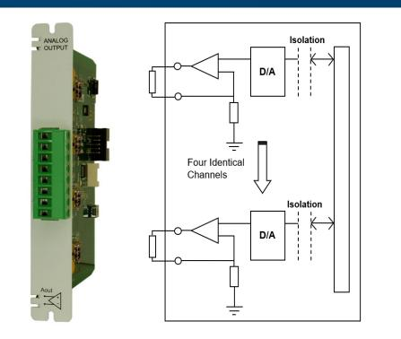
The MAO-010 is a 4-channel individually isolated analogue output module. The current output range is  $\pm 20$ mA with a build option providing for  $\pm 10$ VDC outputs. Both the current and voltage card variants feature 20% overrange.
