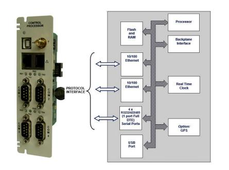
The MCP-012 module provides a range of communication options including Ethernet and four configurable RS-232 / RS-485 ports. It supports industry standard protocols including IEC61850, DNP3, IEC104, IEC101, IEC103 and Modbus.
