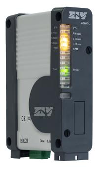
The 4GWC-gateway forms part of a remote management system with automatic meter reading (AMR) through the low voltage network (Power Line Communication or PLC).
