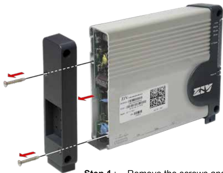
Step 1 : Remove the screws and extract the rear cover.
