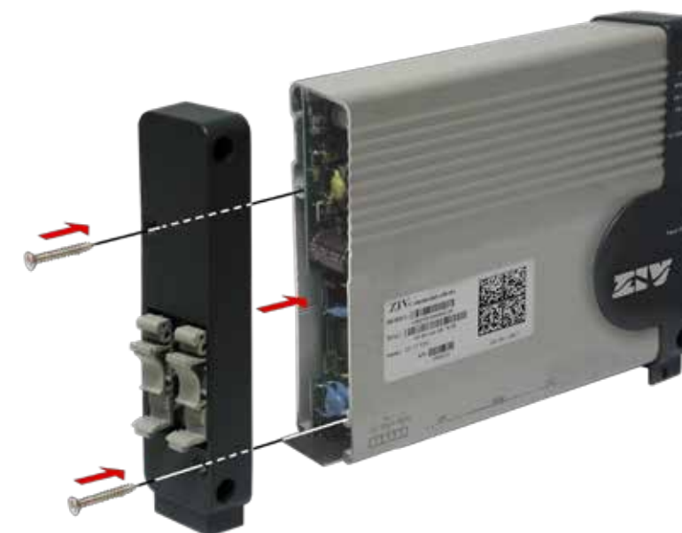
Step 4 : Place the rear cover, by securing it with the screws removed in step 1.
