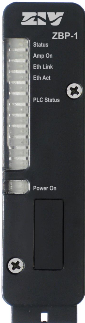
FIGURE 9 Detail of the different LEDs of the ZBP-1
