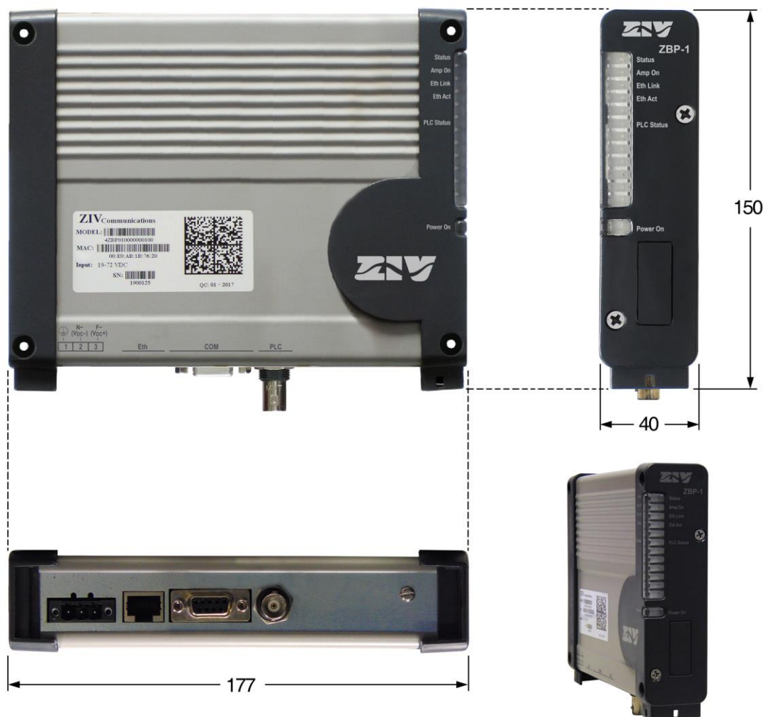
FIGURE 2 Overall dimensions in mm of the ZBP-1
