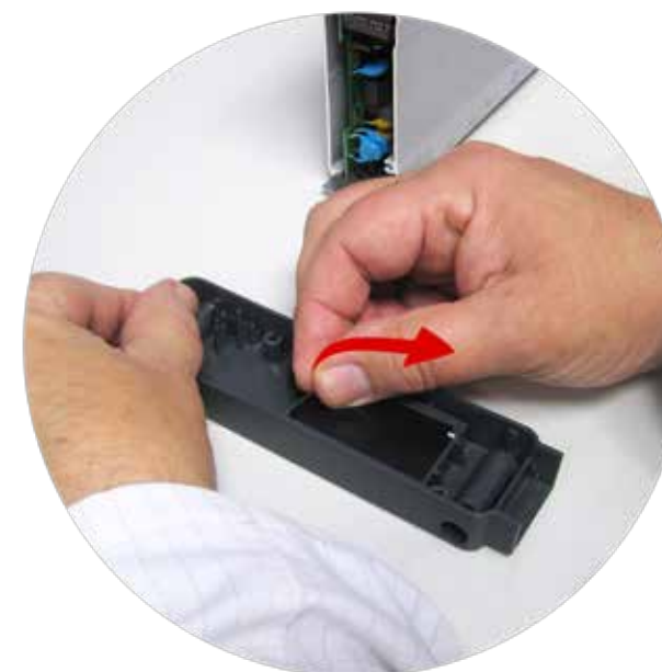
Step 2 : Remove the adhesive strip that secures the holes for screwing the DIN rail accessory.
