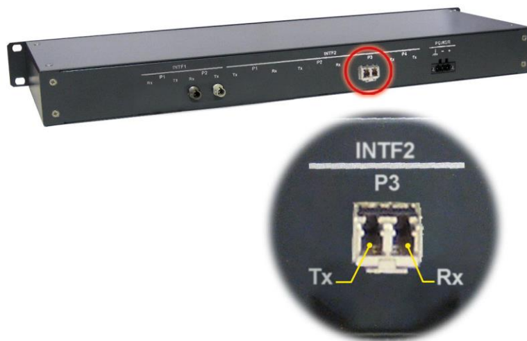
FIGURE 10 C37.94 signals, for SFP bay, of INTF2 (P3 position)
