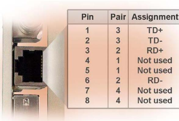
In the eight 10/100Base-Tx ports that admit the PoE power-supply option (1 to 4 of block 1 and 1 to 4 of block 2), pair 1 is used for the  $V_{DCPoE+}$  connection, and pair 4 is used for the  $V_{DCPoE-}$  connection.
