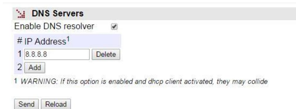
As indicated in the warning of the figure, it must be taken into account that the simultaneous configuration of the DNS servers together with interfaces operating in DHCP mode may imply an incorrect final configuration, given that it is quite typical that the DHCP setup should also include the DNS servers.
