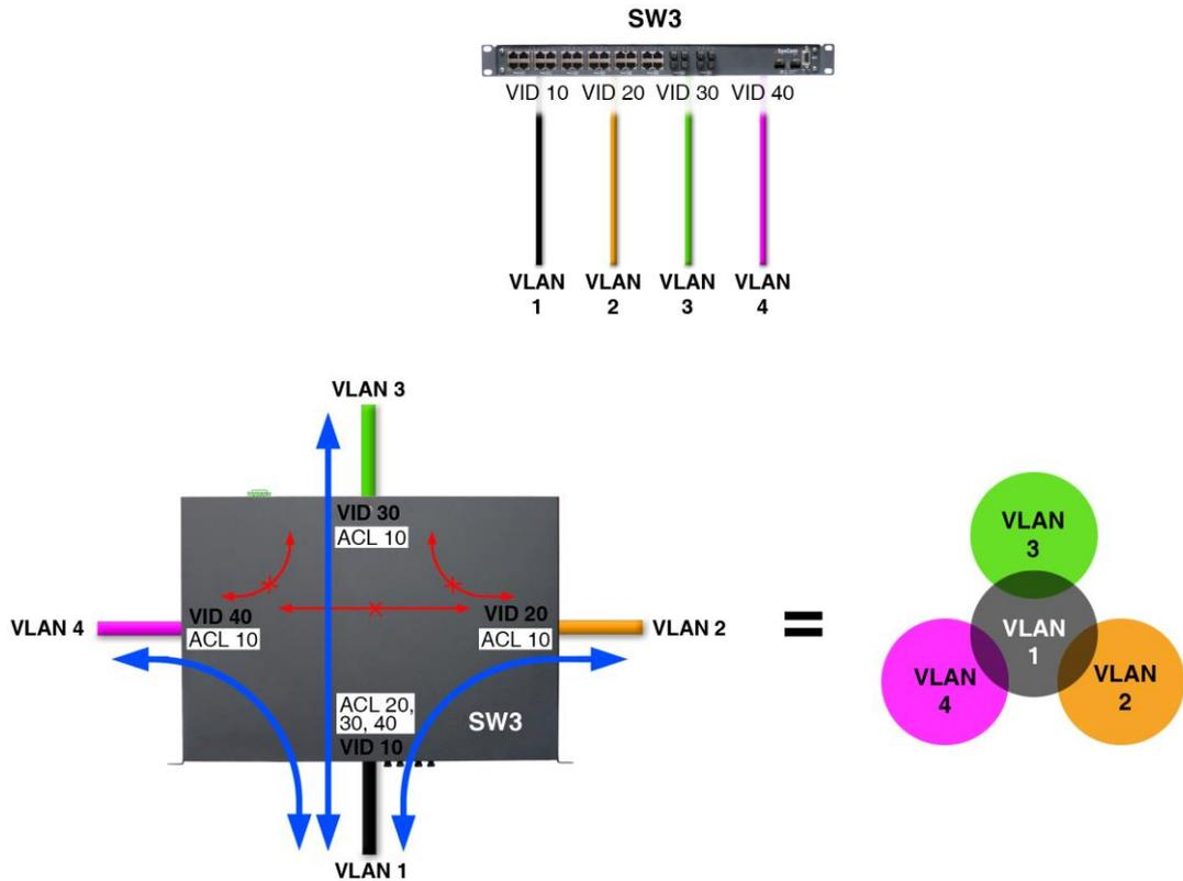
**4 VLANs with common ports and UNTAGGED clients = OVERLAPPING ENABLE ACTIVATED**
