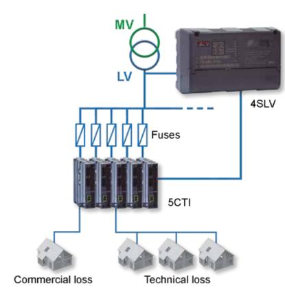
Two ways of determining the LV feeder to which each meter is connected
