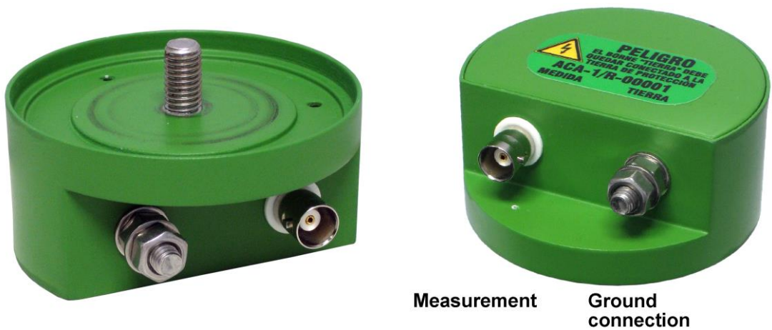
Figure 4 Detail of the APMR-1/R block connections
