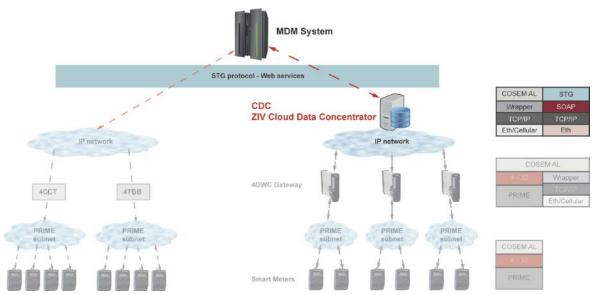
The Cloud Data Concentrator is a key component for AMI deployments as it allows 100% coverage for PLC smart meters.
