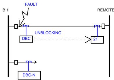
FIGURE 5 – Line end-point protection.
