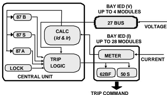
FIGURE 1 – DBN Protection Modules
