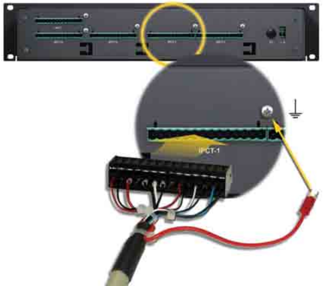
FIGURE 3 Detail of the earth-connection screws
