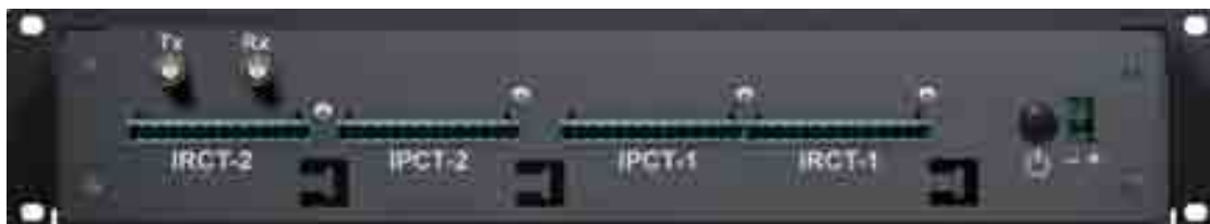
FIGURE 8 Terminal connectors for external connections when the line interface is digital at 2 Mbit/s
