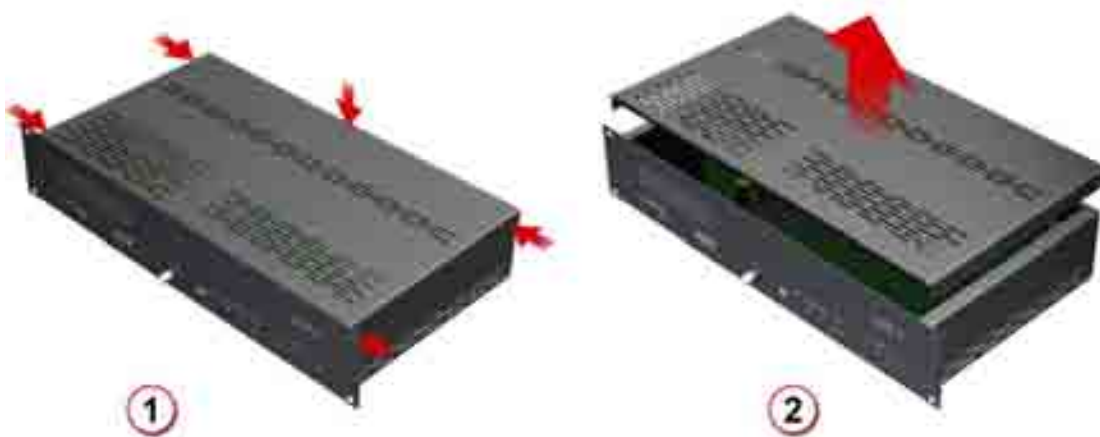
FIGURE 23 How to extract the top cover
