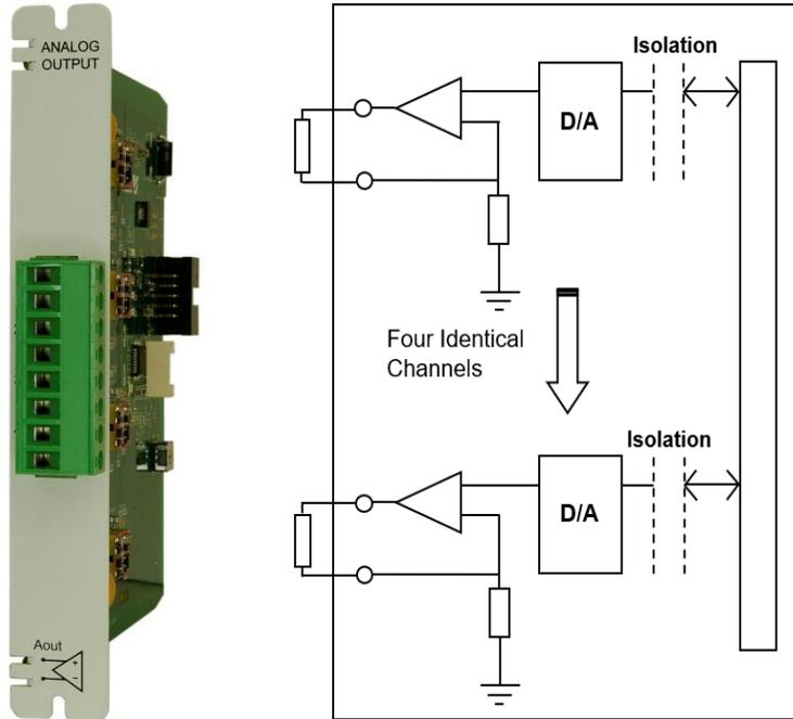
The MAO-010 is a 4-channel individually isolated analogue output module. The current output range is  $\pm 20\text{mA}$  with a build option providing for  $\pm 10\text{VDC}$  outputs. Both the current and voltage card variants feature 20% overrange.
