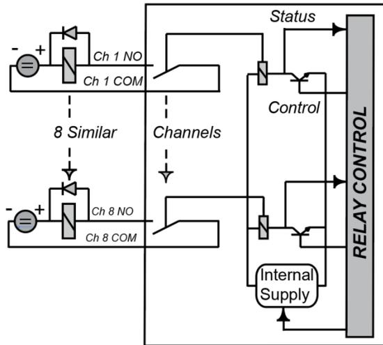
The MDO is an 8 channel digital output module with a single normally open contact per channel. Suitable for 125VDC operation
