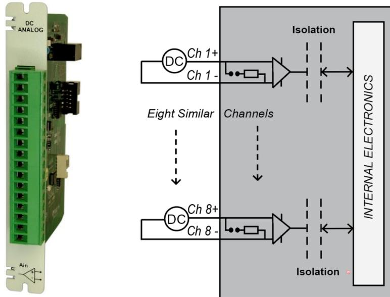
The MAI is an 8 channel DC analogue input module which provides the measurement options for 0-1V, 0-10V,  $\pm 1V$ ,  $\pm 5V$ ,  $\pm 10V$ ,  $\pm 20mA$  and 4-20mA.
