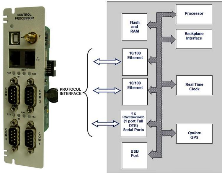
The MCP-012 module provides a range of communication options including Ethernet and four configurable RS-232 / RS-485 ports. It supports industry standard protocols including IEC61850, DNP3, IEC104, IEC101, IEC103 and Modbus.
