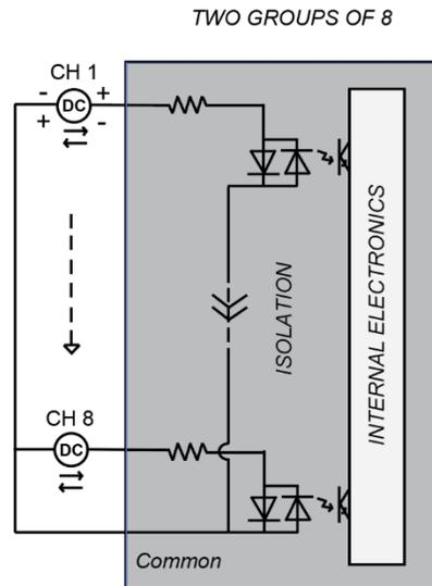
The MDI digital input module has 16 digital input channels organized as two groups of 8 with respective commons. It accepts bidirectional Voltage-Driven inputs and provides optically isolated input channels with field voltage ranges from 18 to 72V DC and 36 to 150V DC.
